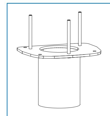
The adapter requires a concrete base with screw tightening for a column of a diameter of 115 mm. The adapter must be securely mounted with the mounting screws of the concrete base. Tightening torque may vary depending on the concrete base.
