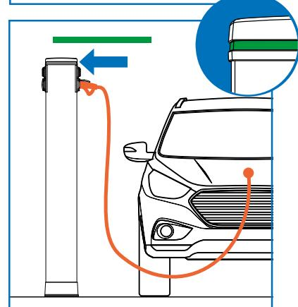
when the cable is first disconnected from the vehicle. This also unlocks the charging station lock.
