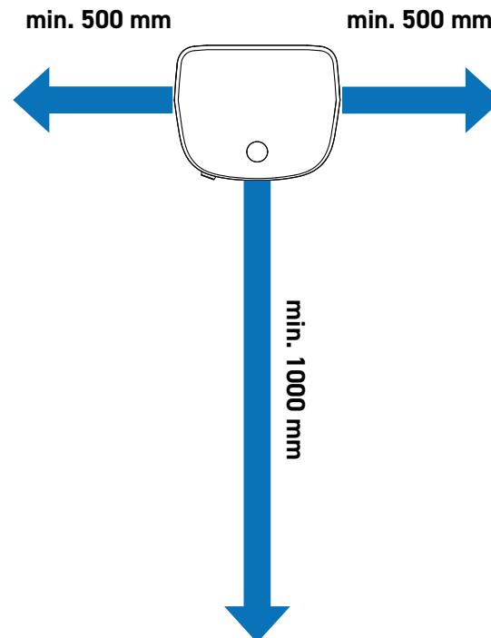
**Please note!** It is not recommended to mount the station in direct sunlight or any other warm place. Excessive inside temperature of the station will limit the charging current.
