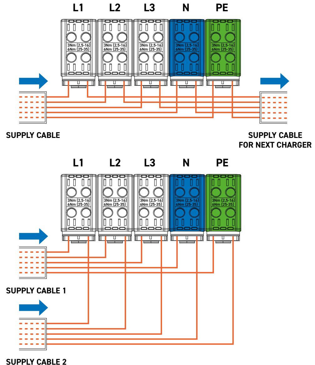
Strip the conductors of the supply cable to a length of 15 mm.
