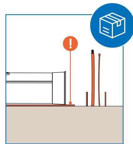
Lay the station on its back with the bottom of the station close to the ground-mounted attachments and supply cables. Please note that the position must be protected against dents and scratches before placing it on its back. You can use, for example, the station's packaging as protection.
