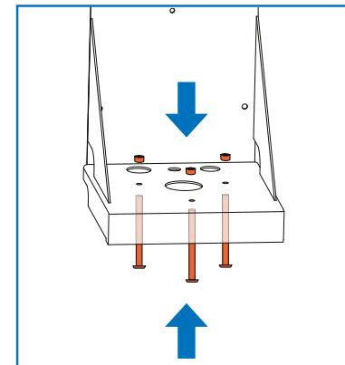
The base is wall-mounted with the bottom of the base resting against the ground.
