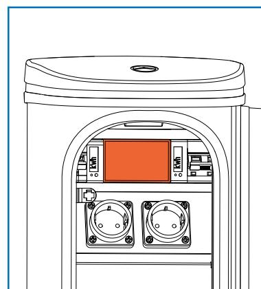
**Please note! Remember to close the station door. An open door may collect dirt and water inside the station.**
