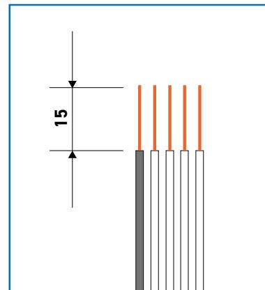
Make the connection. The tightening torque of the supply connector is 3 Nm (2.5...16 mm<sup>2</sup>) or 6 Nm (2.5...35 mm<sup>2</sup>). Make sure that the loop of wires does not rise too high. Wires that rise too high may make it difficult for the frame to settle in place or the wires to be compressed. There are height markings on the mounting plate to help.
