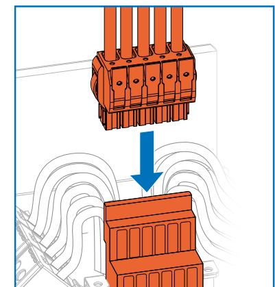
Then lower the station component into its place, aligning the hem of the contact protection in the station component with the groove in the bottom cup. Make sure that the station component is properly seated.
