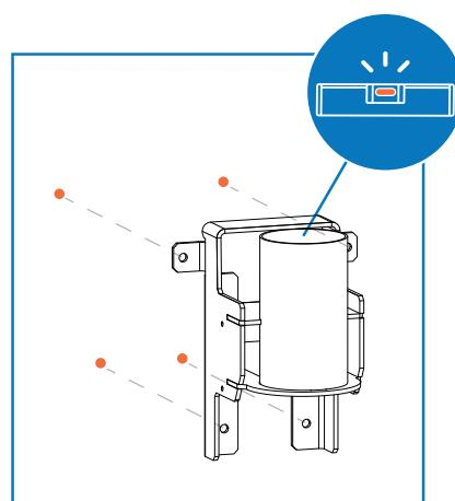
The station is attached to the wall mount as in the column mounting procedure. See section 5.2.1. Supply cable.
