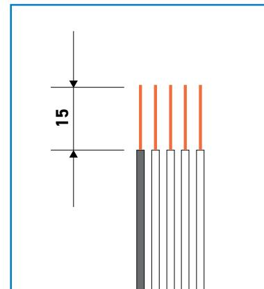
Make the connection. The tightening torque of the supply connector is 3 Nm (2.5...16 mm<sup>2</sup>) or 6 Nm (2.5...35 mm<sup>2</sup>). Make sure that the conductors' loop does not rise above the bottom cup mounting plate, as the frame is lowered to this height and conductors may get pinched.
