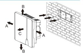
Fig. 8: Drilling holes for wall mounting
