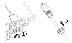
Fig. 28: insert the network cab
