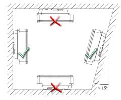
Fig. 5: Permissible installation location
