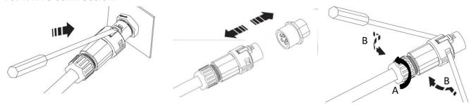
Fig. 39: Detach the AC connection plug Fig. 40: Disconnect AC connection plug Fig. 41: Release the cable
