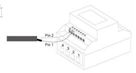
Fig. 33 Connect Network cable
