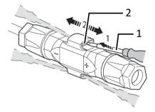
Fig. 42: Unplugging the plug connector
