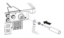
Fig. 25: connect the grounding
