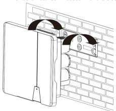
Fig. 10: Mounting the inverter to the wall bracket
