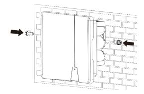
Fig. 12: Fixing the inverter
