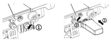
Fig. 26: Connect the communication device
