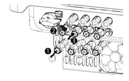
Fig. 43: Insert DC plug connection
